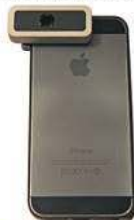
Figure 1 - Picture of the prototype magnetically attached to an iPhone 5 (Apple, Cupertino, CA).
