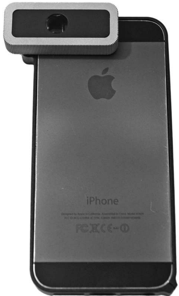
FIGURE 1. Depiction of the D-Eye prototype magnetically attached to the smartphone.
